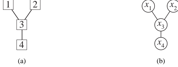
Figure 3: (a) Undirected communication topology \mathcal{G} considered in the example scenario. (b) Illustration of the corresponding Markov Random Field \mathcal{G}_X subject to estimation by the decentralized estimation network.
